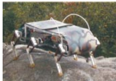
Figure 1: RHex with 4-bar legs in a natural setting.
