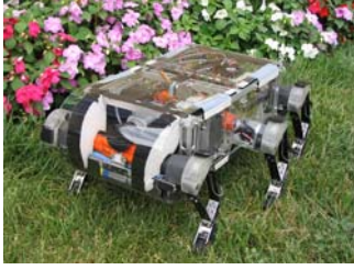
Fig. 1. Left: RHex with 4-bar leg equipped with strain-based leg configuration sensor stands on the meadow; Right: Four consecutive intervals during the i^{th} jogging stride, C(i) .
