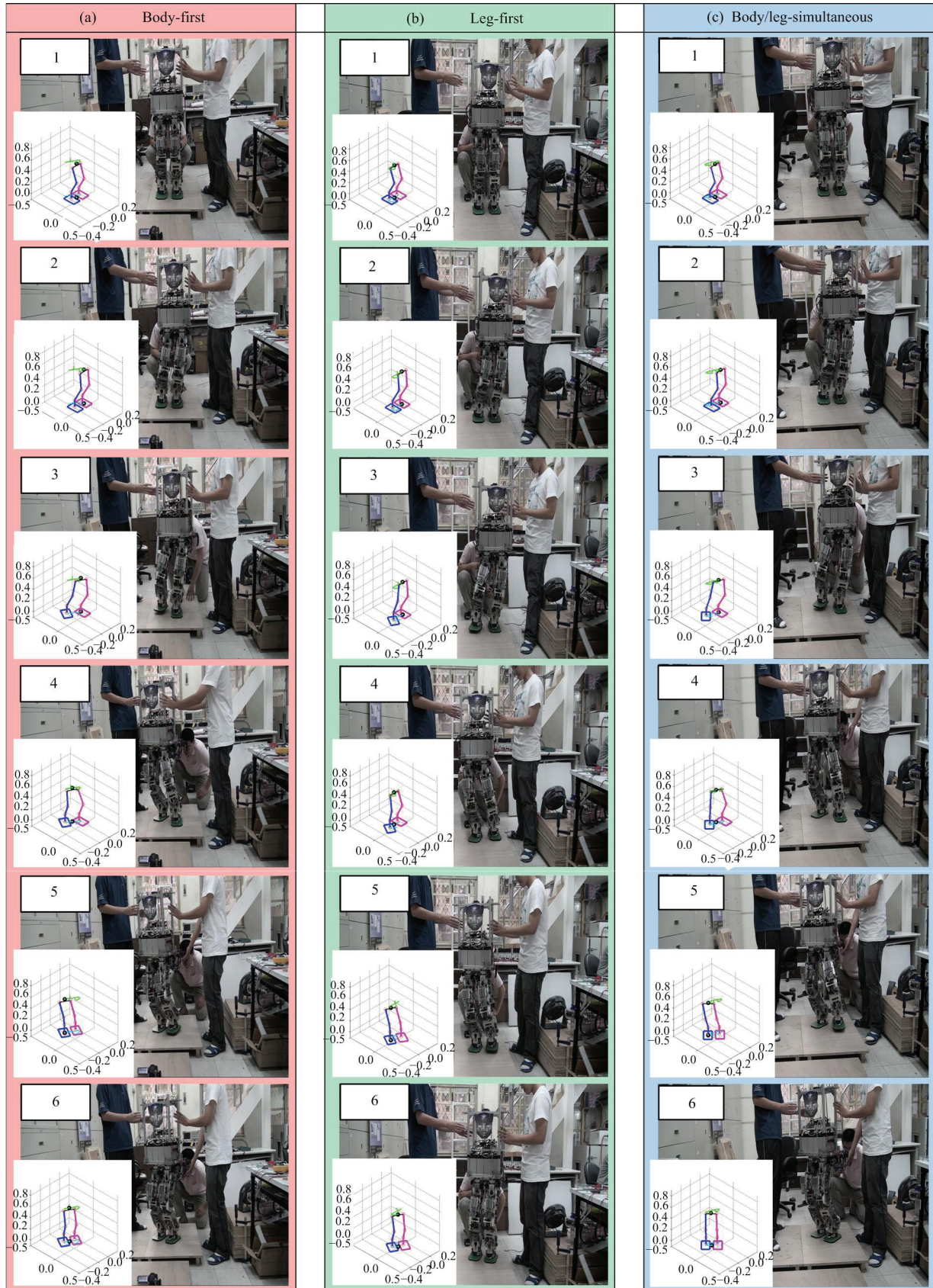
Fig. 10 Sequential snapshots of the robot performing three different methods of turning in place. (a) Body-first; (b) leg-first; (c) body/leg-simultaneous. The robot configurations shown in snapshots 1–6 correspond to the motion steps from (b) to (g) discussed in section 2.1 and also shown in Fig. 3.
