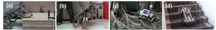
Fig. 9. Robot operated in various scenarios: (a) step crossing, (b) bar crossing, (c) natural rough terrain walking, and (d) stair climbing.
